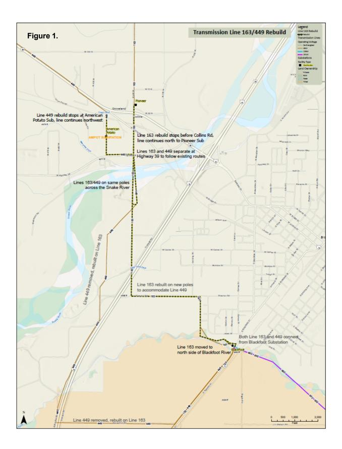
Idaho Power plans to begin construction in 2025 and complete construction in early 2026. Idaho Power will install new poles and string wire in segments, to minimize interruptions to traffic and electrical service. As part of the construction, Idaho Power will remove old poles and rehabilitates any damages. Due to the nature of project schedules and material procurement, Idaho Power requests Planning and Zoning Commission approval for the maximum 10-year period, per Bingham County Code §10-8-5.
